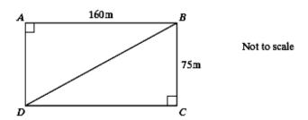
The length of the field, AB = 160m. The width of the field, BC = 75m. Calculate the length of the diagonal BD. Give your answer to a suitable **degree of accuracy**.
