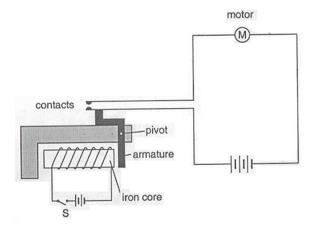
Label the poles of the iron core on the diagram when the switch **S** is closed.
