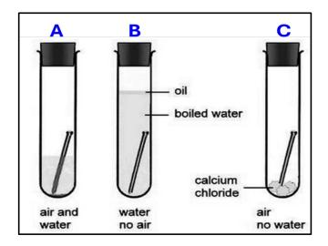
39. Rusting is a serious and costly problem Rust weakens steel and iron structures. The process of rusting in iron occurs under specific conditions illustrated in the diagram above.
