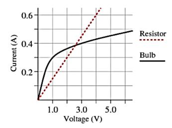
In term of resistance (R), describe and interpret the behavior of the bulb relative to the resistor at different voltages. (HINT: Use R = V/I)
